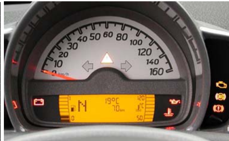
Instrument cluster with multifunctional display. Includes a clock, fuel-level, coolant-level, residual fuel, service interval, and trip mileage indicators.
