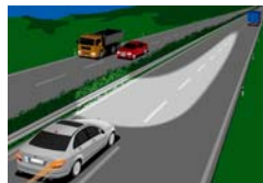
Motorway mode: more even, longer-range light distribution than with con- ventional low-beam head- lamps (small image above)
