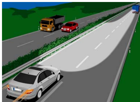
Motorway mode: more even, longer-range light distribution than with con- ventional low-beam head- lamps (small image above)
